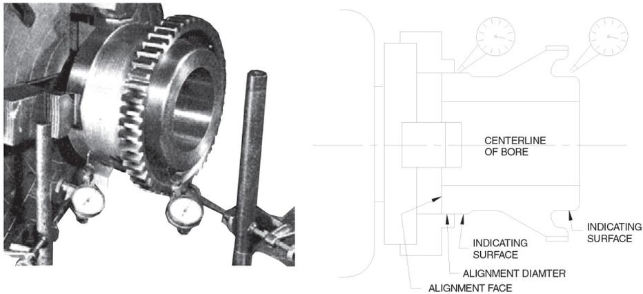
The alignment diameter of the hub should be chucked in the boring lathe and dial
