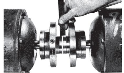
**Recheck angular alignment and hub separation.**
